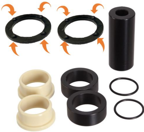
New „crush washer“ mounting hardware – eliminating side to side play
